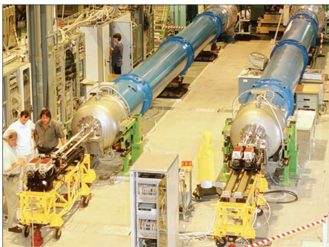
The first two LHC dipoles undergoing tests on the cryogenic benches in the SM18 test facility at CERN's Meyrin site in 2001.
