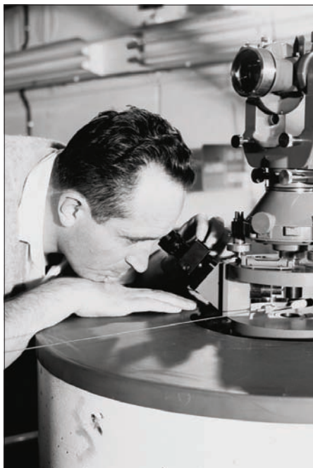
Gervaise taking measurements with invar wire and a theodolite on a pillar at the PS.
