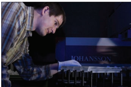
Igor Tarasov inserting the last batch of the CMS lead tungstate crystals into one of the machines that was developed to measure 67 different parameters for each crystal.
