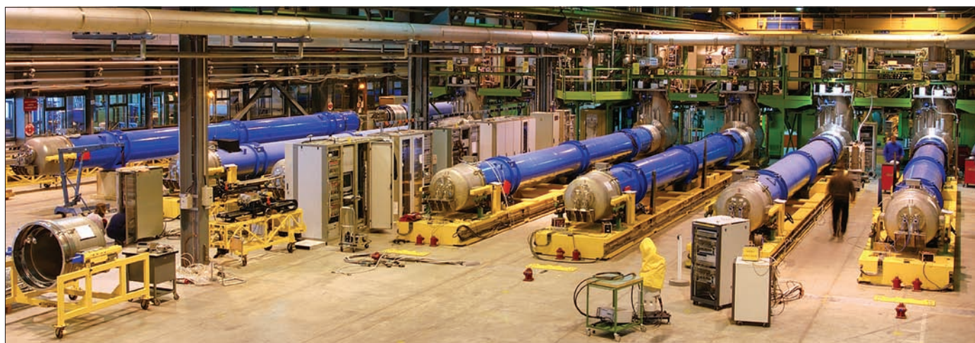
Several dipole magnets in various stages of cold testing in March 2004. The remaining test benches, which make up the full complement of 12, are located on the other side of the gantry, which contains the cryogenic and power systems.
